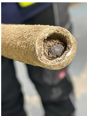
Left: Photo taken at an EfW site demonstrating a typical failure mode of high-temperature thermometers. Shown is the cracking and failure of an alumina ceramic thermowell.
